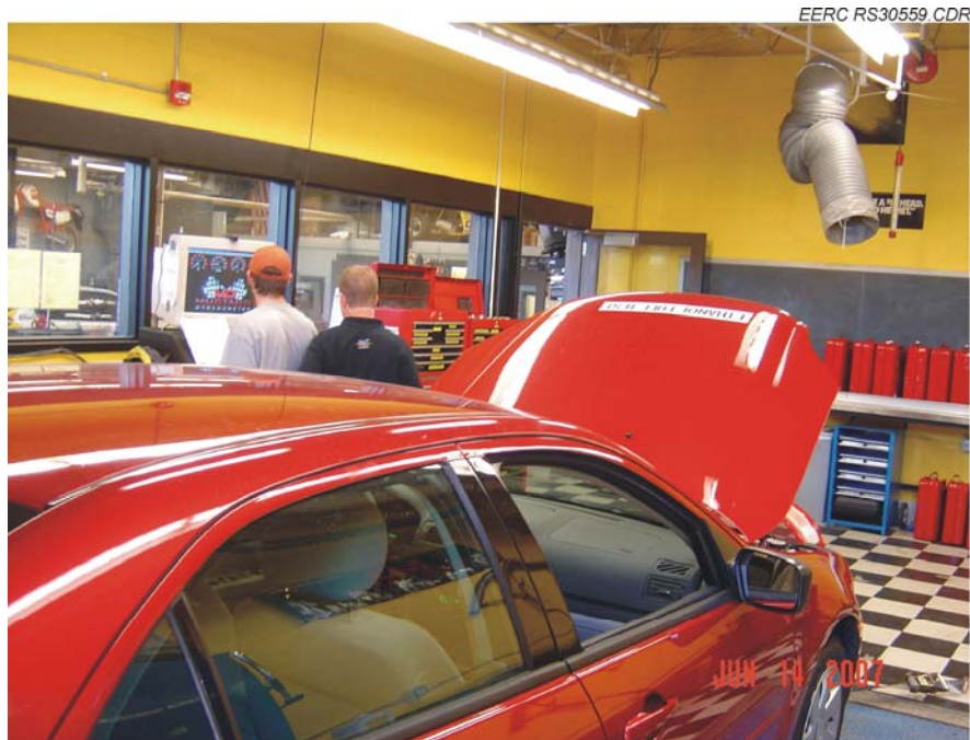
Figure 5. Mustang chassis dynamometer.
