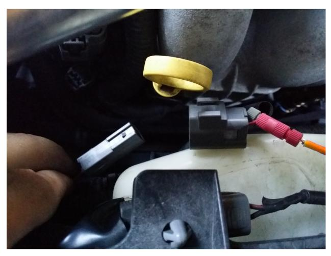
Next, locate the larger black wire that is coming out of terminal 3 of the relay. To double check, disconnect the relay from its socket and look inside the relay itself to see the terminal numbers written next to the blades of the relay. Match this terminal to the corresponding terminal when plugged in on the socket which should result in the larger of the two black wires coming out of the relay harness.
