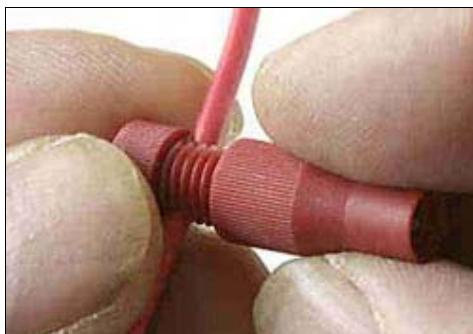
Here the tap is started carefully onto the threads of the large cap. Make sure the pin is centred on the wire when the pin contacts the wire. Keep the Posi-Tap straight to do this.
