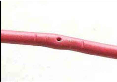
Tapped wire after removal.
