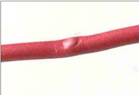
Backside of tapped wire.
