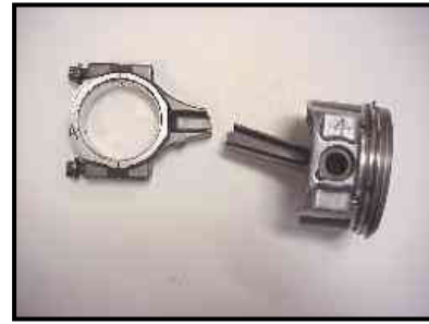
Figure 8 Rod Failure in Tension
