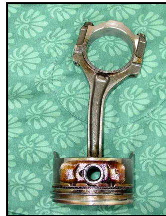
Figure 10 Rod Failure in Compression
