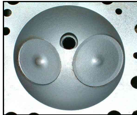
Figure 1 Hemispherical Combustion Chamber
